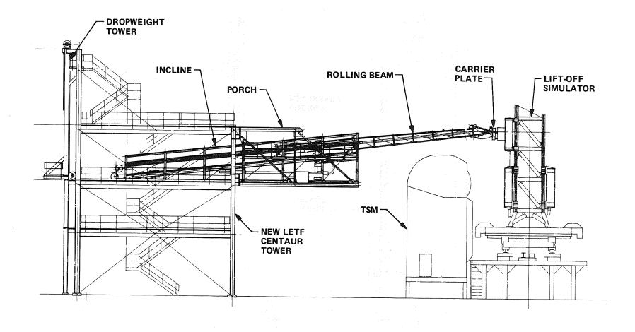
Figure 9. Launch Equipment Test Facility-STS/Centaur Rolling Beam Umbilical System Installation
